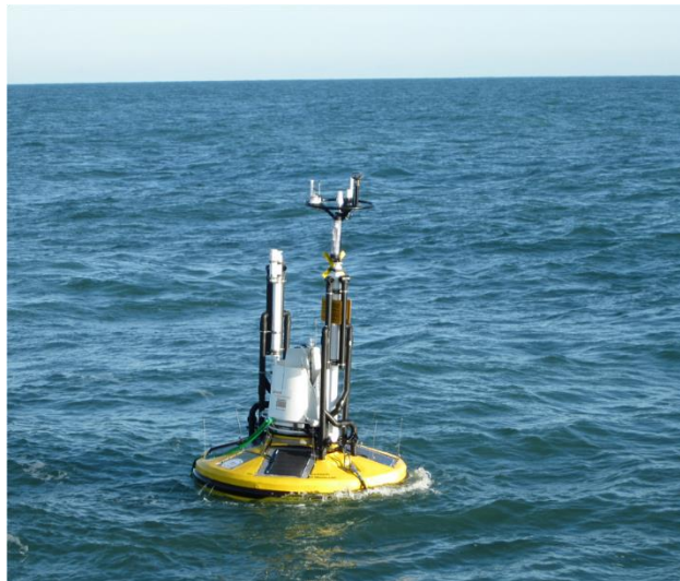
Figure 6 Seawatch wind lidar buoy (photo provided by Fugro).
